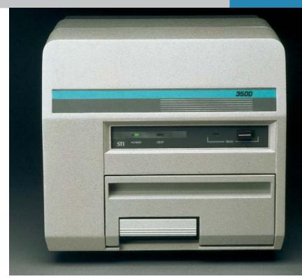
The Harshaw 3500 includes a sample drawer for a single element TLD dosimeter, a linear, programmable heating system and a cooled photomultiplier tube with associated electronics to measure the TL light output. The manually-operated Harshaw 3500 is used in medical physics, health physics, materials research, food irradiation and industrial applications.
