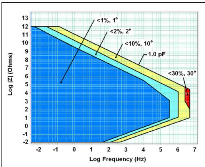
Typical results for PARSTAT 4000 with standard 2m cable, potentiostatic mode, and Faraday Cage
