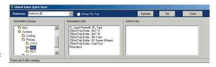
Value. The Quick Start module is a thick toolbar that acts as the centralized launch pad for initiating automation routines and accessing Sample and QA administration modules. Jobs are logically grouped in folders similar to Windows Explorer and launched with a single mouse click. Quick Start also keeps track of active Jobs making it easy to determine when a detector is available for a new sample.
