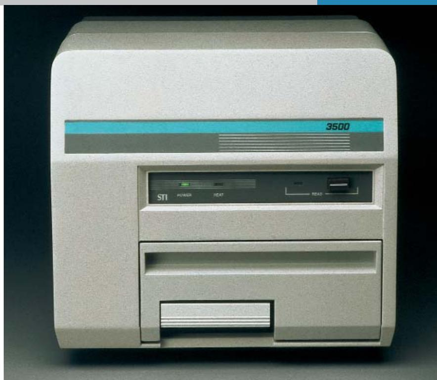
The Harshaw 3500 includes a sample drawer for a single element TLD dosimeter, a linear, programmable heating system and a cooled photomultiplier tube with associated electronics to measure the TL light output. The manually-operated Harshaw 3500 is used in medical physics, health physics, materials research, food irradiation and industrial applications.
